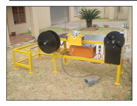
The semi automated bench coiling machine is suitable for warehouses and industries where repetitive lengths of cable, rope, hose and similar materials need to be cut. This machine enables simultaneous functions of feeding, measuring and coiling of material as a single operation. Standard 220V power supply is required for operation.
